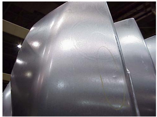
Fig. 3 Sliver imprint into the panel surface
